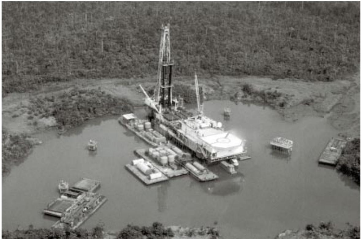
*Barge Rig 74 drilling in Nigeria*
